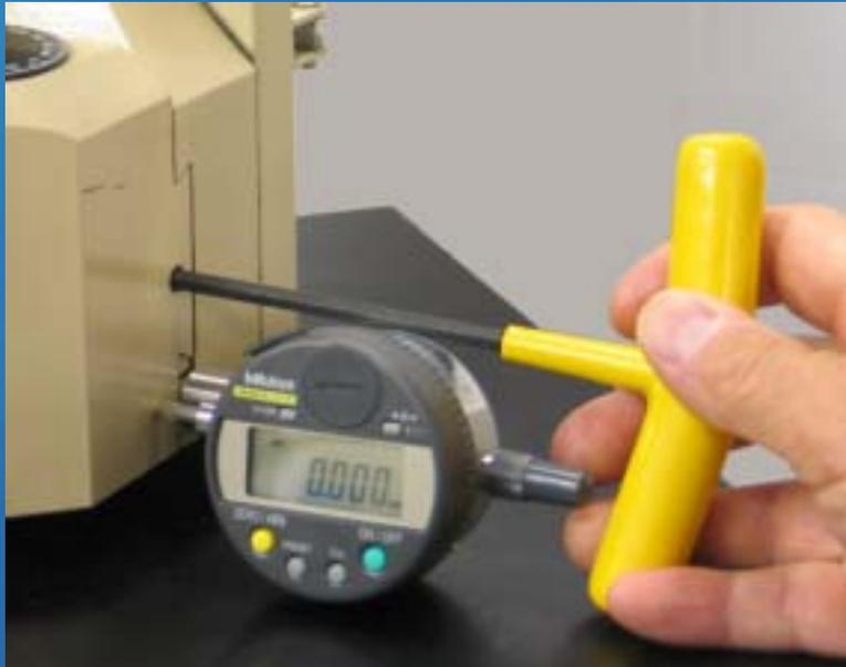
The lower chuck, which we will call the "X" axis, carries the lens, and is adjusted along a zero to 180 axis by turning the lead screw as indicated in the photo with the provided t-wrench.
