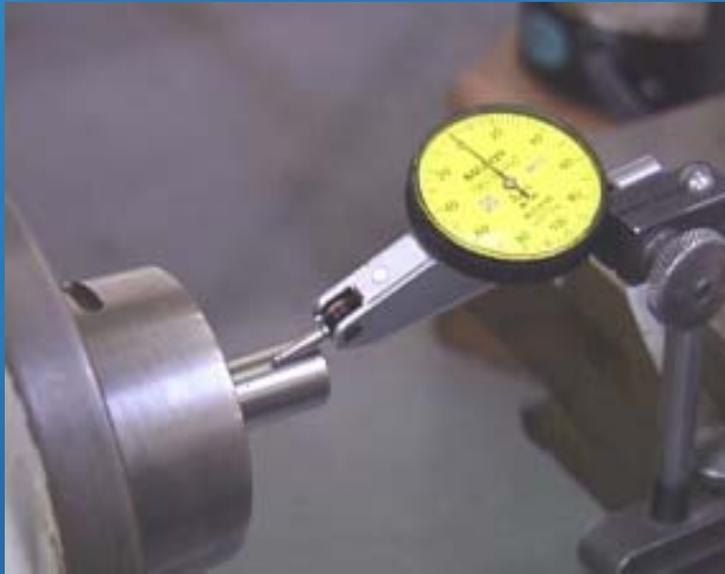
After thoroughly cleaning the Lathe collet, lock the gage pin in to the depth of a normal arbor. Move the dial indicator into place. Set it to zero, then rotate the spindle to see how much eccentricity
