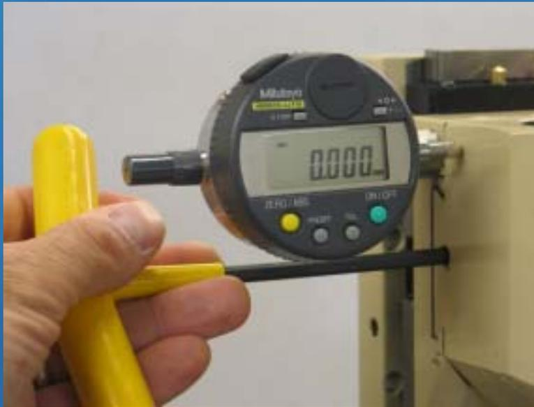
According to our chart we turn the arbor chuck adjustment set screw counter clockwise to move the arbor .011mm.
