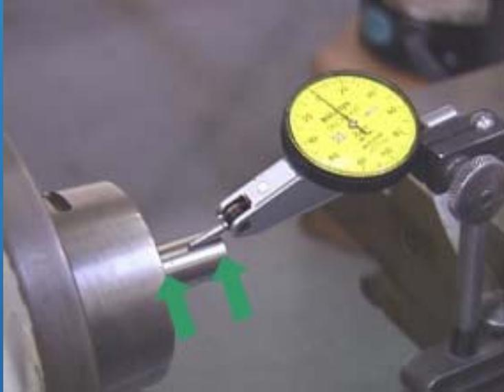
Also check the gage pin at the face of the collet. And then again at the outer end. This may reveal an angular component to runout. Your collet must be holding the gage pin to within .005mm and parallel to the
